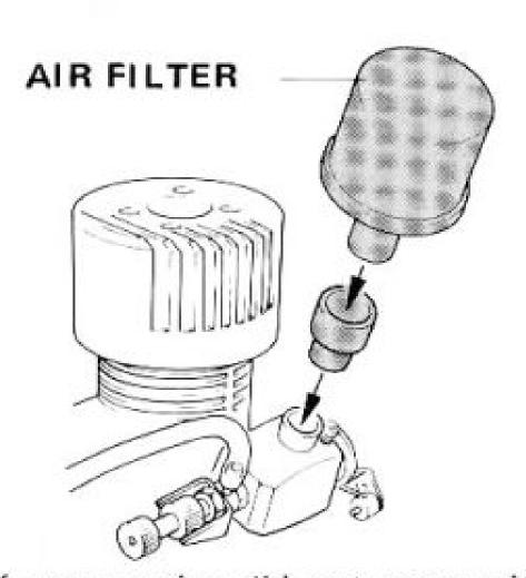
If your engine did not come with an air filter, you must use one! If not, dust and other contaminants will damage your engine. The Kyosho CB-110 Air Filter should do the job for most engines.
